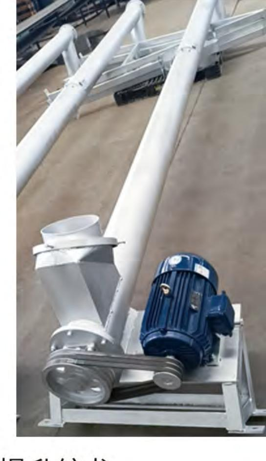
提升绞龙 Lifting screw feed conveyor
